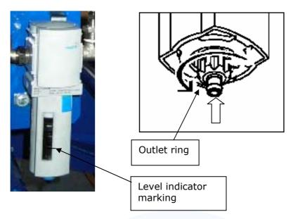
In case of less air flow as mentioned in the paragraph above, replace the filter of the water separator as following:
